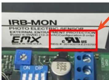
UL Recognized This UL logo indicates that the component, in this case an EMX photo eye, was tested by UL and met the UL 325 standard for photo eyes.
