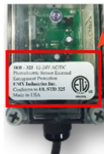
ETL Listed This circular ETL LOGO with a registration number below indicates that the component, in this case an EMX photo eye, was tested by Intertek and met the UL 325 standard for photo eyes.
